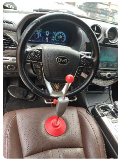
Figure 3.1-1 Fitting the steering wheel lock
