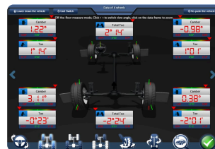
Figure 4.3-4 Four-wheel data screen in lift mode
