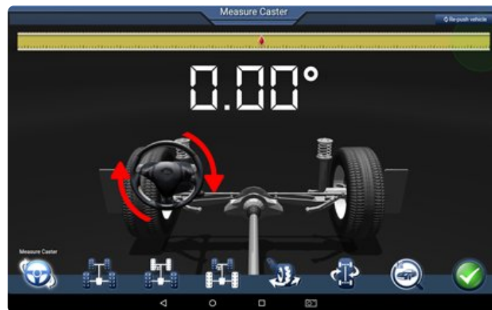
Figure 4.2.3-1 Caster measurement screen
